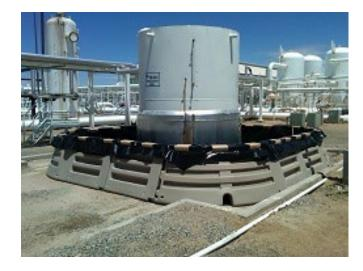
The Stinger PolyBerm is a hybrid containment system that takes advantage of the strength of molded plastic and blends it with the portability of industrial fabrics. Combined with simple setup, these features make this containment system the best option for large tanks and transformers.
